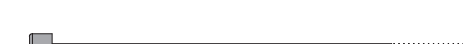
94398 Cap Head Screw M3x55mm Inbusschraube M3x55mm Vis tête cylindrique M3x55mm キャップネジ M3x55mm
